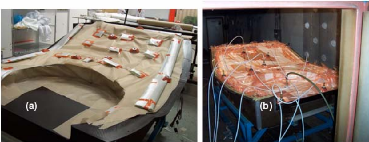
Fig. 5 (a) The bleeder material is placed and (b) the mold is bagged and placed into the oven.
